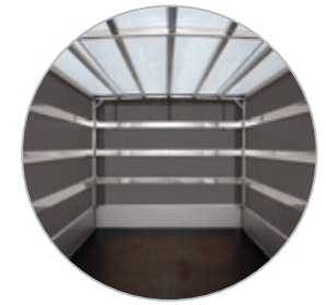
Accessorie: High cover provided with light transmitting tarpaulin
